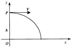
(a) A particle is projected horizontally from a point P, h metres above O, with A velocity of V metres per second. The equation of motion of the particle are,  $\ddot{x} = 0$  &  $\ddot{y} = -g$
